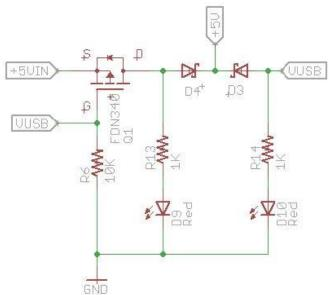
Once you put this circuit on to a PC board, you could legitimately place a plus sign on the anodes of D3 and D4, and another on their cathodes.
