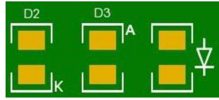
"K", is used because "C" could imply that the spot wants a capacitor. An "A" adjacent to the Anode on the board works too, though it's less commonly used. If you are producing your board without silkscreen, you can put the mark in the copper layer, or submit a clear assembly drawing with the other board files.
